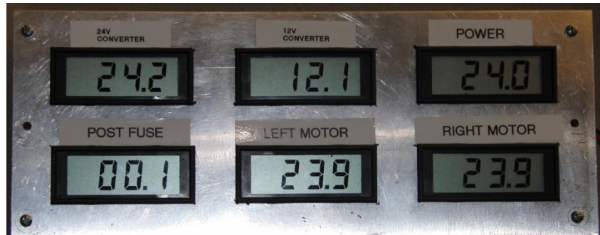
Figure 3.1: Voltage Health Monitoring System
