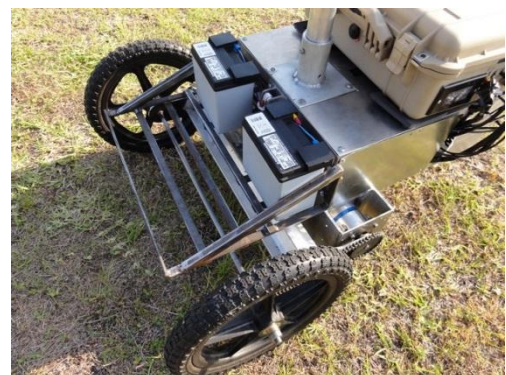
Figure 7.2: MagnaPower AGM Batteries
